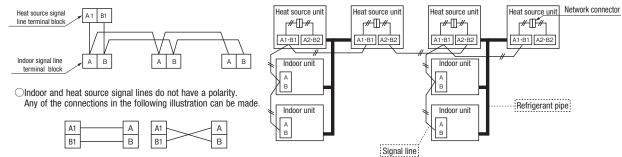
(3) The signal lines can also be connected using the method shown below.
