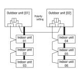
· Within a refrigerant system, indoor units are assigned addresses in the order they are recognized by the outdoor unit. Therefore, they are not necessarily assigned addresses in order from the nearest to the outdoor unit first as depicted in drawings above.
