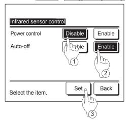
The Infrared sensor control screen and contents of the current settings are displayed.
