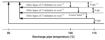
Notes (1) When the discharge pipe temperature is in the range of 105-115°C, the speed is reduced by 4 rps.
