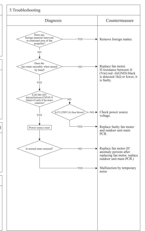
Note: When E48 error occurs, in almost cases F3 fuse (1A) on the outdoor unit main PCB is blown. There are a lot of cases that fuse is blown and E48 occurs due to defective fan motor. And even though only the outdoor unit main PCB ( or fuse) is replaced, another trouble could occur. Therefore when fuse is blown, check whether the fan motor is OK or not.
