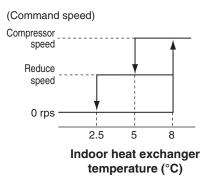
(1) When the indoor heat exchanger temperature is in the range of 2.5–5°C, the speed is reduced by 4 rps at each 20 seconds.
