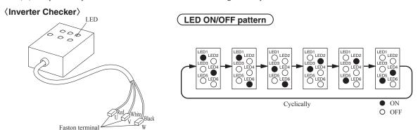
Connect to the terminal of the wires which are disconnected from compressor.
