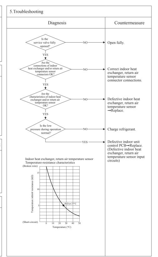
Note: When the compressor speed is 60 rps or under at 5 minutes after the start of compressor or the completion of defrost operation, the low refrigerant protection control judges, by detecting the difference between the indoor heat exchanger temperature (Thi-R) and the indoor return air temperature (Thi-A), that it is in the state of gas leakage, and stops the compressor.
