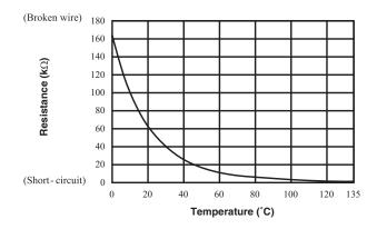
◆ Sensor temperature characteristics [Room temperature, indoor heat exchanger temperature, outdoor heat exchanger temperature, outdoor air temperature outdoor suction pipe temperature]
