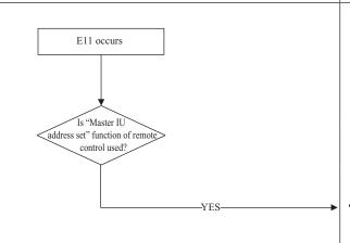
In case the wiring is below and "Mastar IU address set" is used, E11 is appeared.
