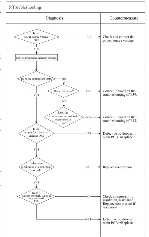
The unit is left for long period without power source or soon after installation, migrated liquid refrigerant may dissolve in the refrigerant oil in the compressor. In such case insulation resistance decreases upto several MΩ or lower. If the electric leakage breaker is activated due to low insulation resistance, check followings.
