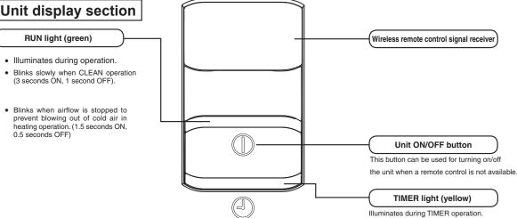
RUN and TIMER lights blink quickly during invalid operation mode
