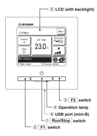
Touch panel system, which is operated by tapping the LCD screen with a finger, is employed for any operations other than the ①Run/Stop, ②F1 and ③F2 switches.
