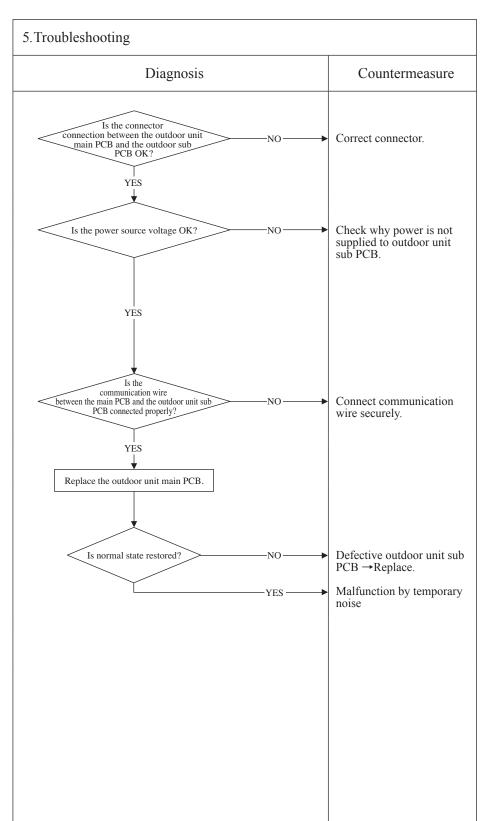
Defective outdoor unit sub PCB→Replace.
