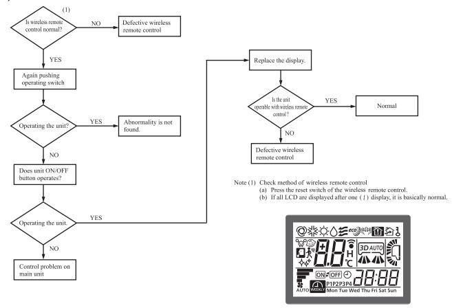
Simplified check method of wireless remote control
