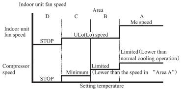
Difference between Setting temperature and return temperature
