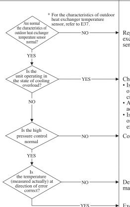
Replace outdoor heat exchanger temperature sensor.
