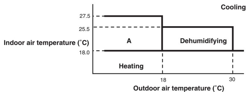
(b) The unit checks the temperature every hour after the start of operation and, if the result of check is not same as the previous operation mode, changes the operation mode.
