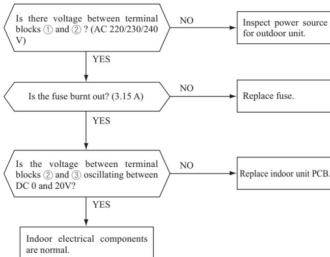
**(b) Indoor fan motor check procedure**
