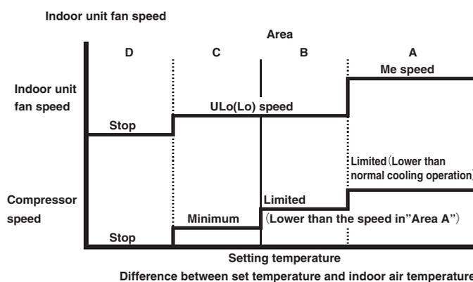
(ii) The indoor unit check the current area by every 5 minutes, and operate by the next checking.
