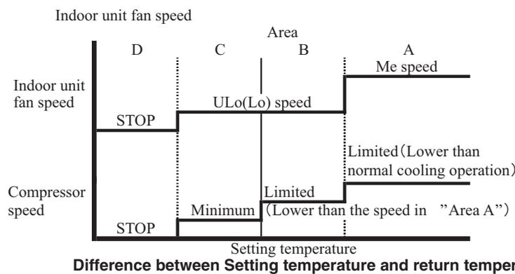
(ii) The indoor unit check the current area by every 5 minutes, and operate by the next checking.
