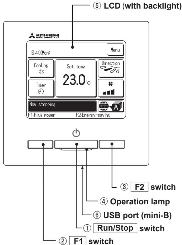
Touch panel system, which is operated by tapping the LCD screen with a finger, is employed for any operations other than the ①Run/Stop, ②F1 and ③F2 switches.
