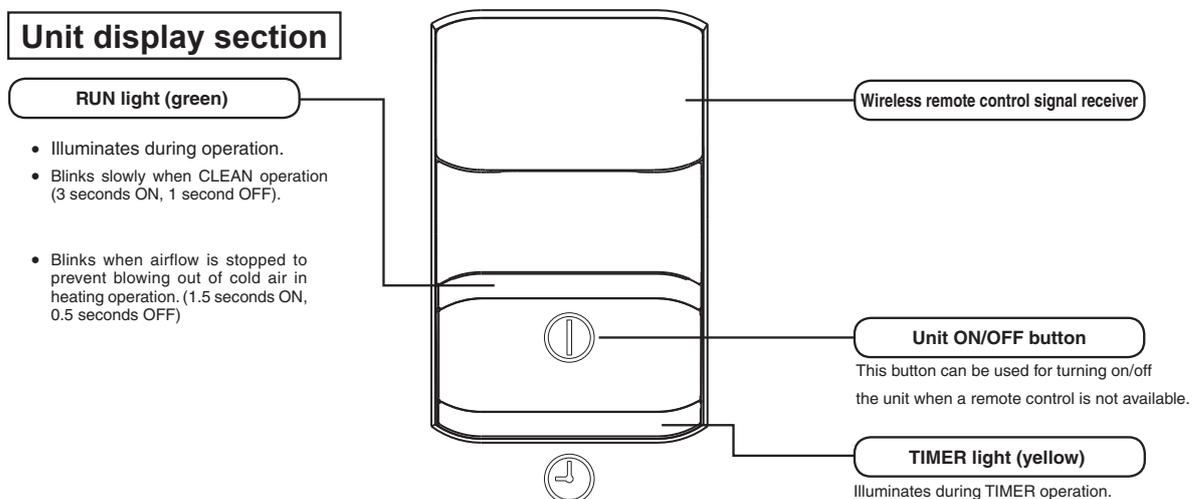
• RUN and TIMER lights blink quickly during invalid operation mode.
