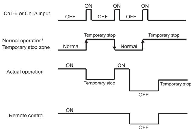
**(23) Selection of cooling/heating external input function**
