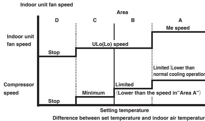
(ii) The indoor unit check the current area by every 5 minutes, and operate by the next checking.
