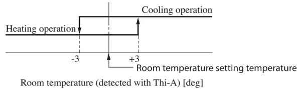
Notes (1) Temperature range of switching cooling/heating mode can be changed by RC-EX3A from  $\pm 1.0 - \pm 4.0$ .
