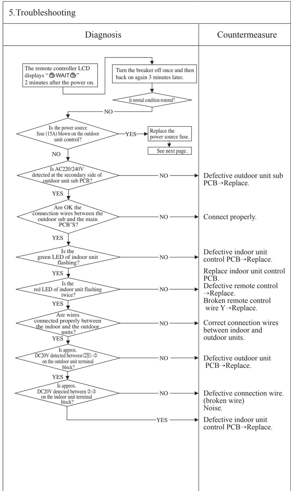
Note: If any anomaly is detected during communication, the error code E5 is displayed. Inspection procedure is same as above. (Excluding matters related to connection) When the power source is reset after the occurrence of E5, the LED will display “🏠WAIT🏠” if the anomaly continues. If the breaker ON/OFF is repeated in a short period of time (within 1 minute), “🏠WAIT🏠” may be displayed. In such occasion, turn the breaker off and wait for 3 minutes.
