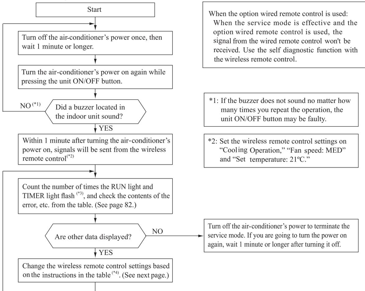
\*3: To count the number of flashes in the service mode, count the number of flashes after the light lights up for 1.5 second initially (start signal). (The time that the light lights up for 1.5 second (start signal) is not counted in the number of flashes.)
