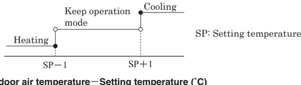
※It can not be changed to heating mode if outdoor air temperature is 28°C or higher.
