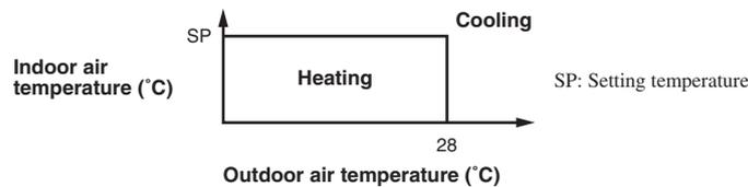
(b) Operation mode is changes when keep cooling and heating thermostat off 20 minutes and be satisfied following conditions. If the setting temperature is changed with the remote control, the operation mode is judged immediately.
