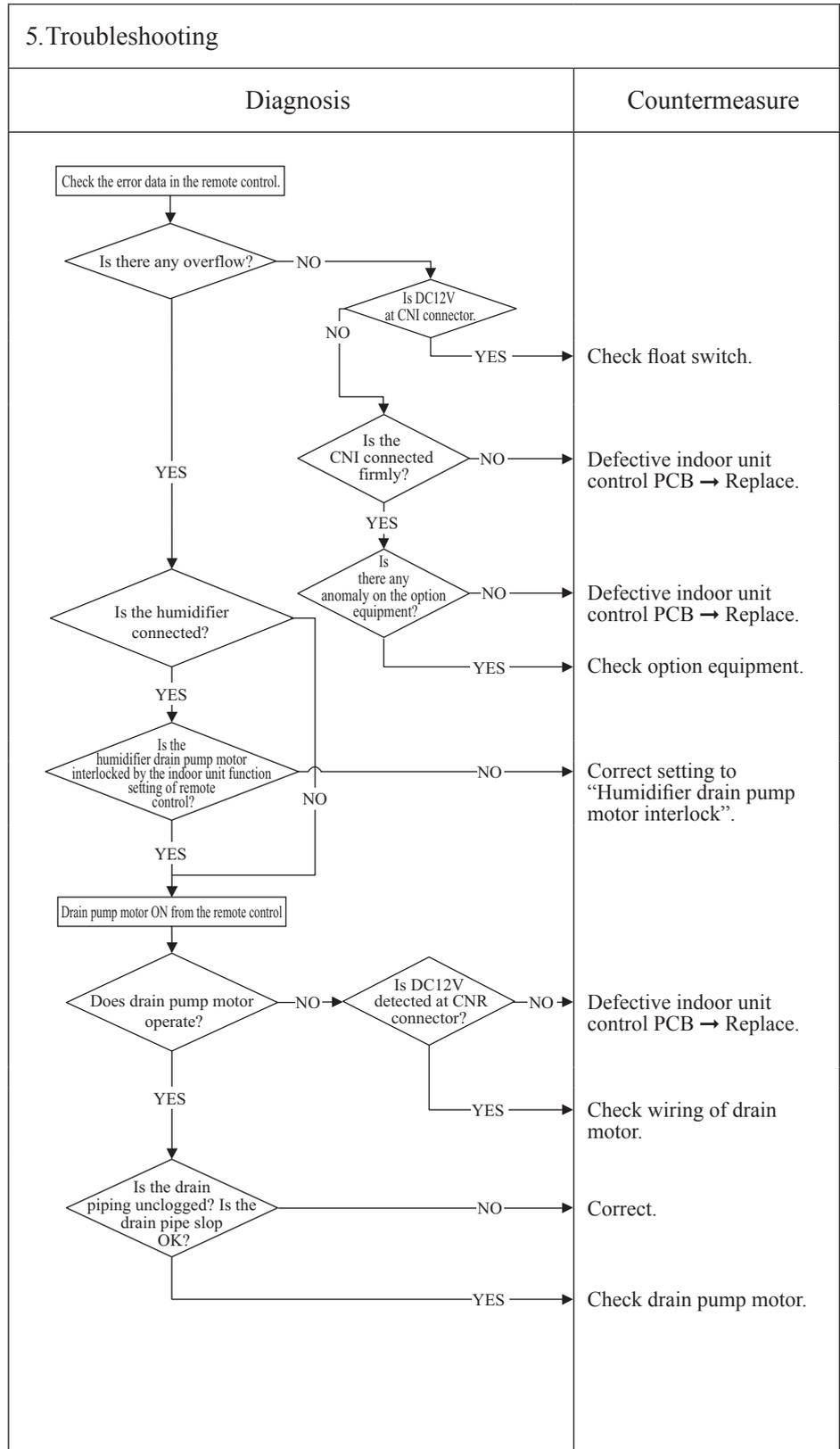
**Note:** When this error occurred at power ON, disconnection of wire or connector of the float switch is suspected. Check and correct it (or replace it, if necessary).
