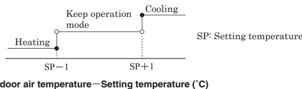
※It can not be changed to heating mode if outdoor air temperature is 28°C or higher.
