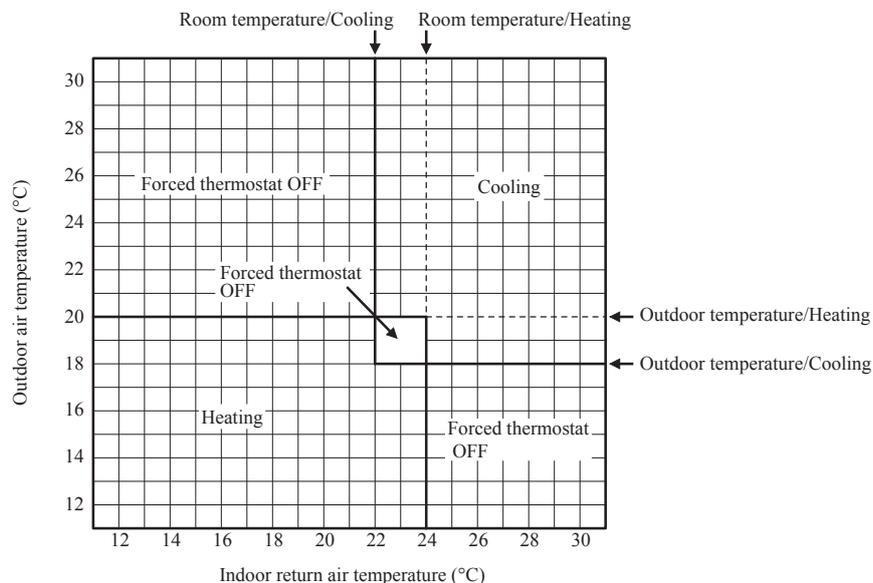
**(2) Operations of functional items during cooling/heating**
