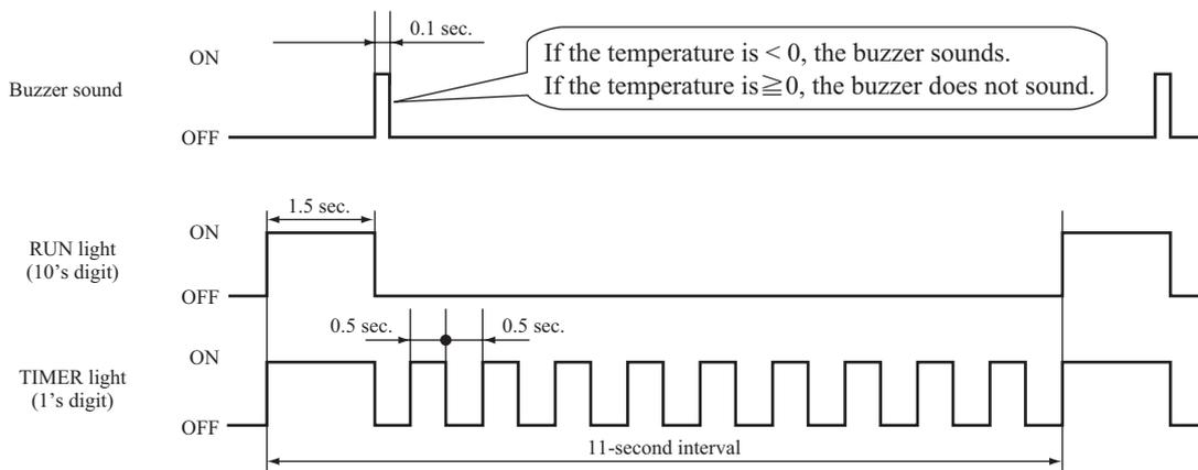
(ii) Discharge pipe temperature sensor temperature
