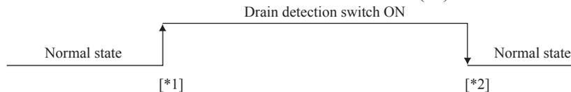
[\*1] Drain detection switch is turned “ON” when the float switch “Open” is detected for 3 seconds continuously in the drain detectable space.
