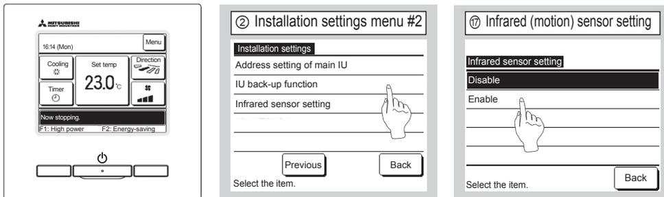
TOP screen **Menu** ⇒ **Energy-saving setting** ⇒ **Infrared sensor control** or **Motion sensor control**
