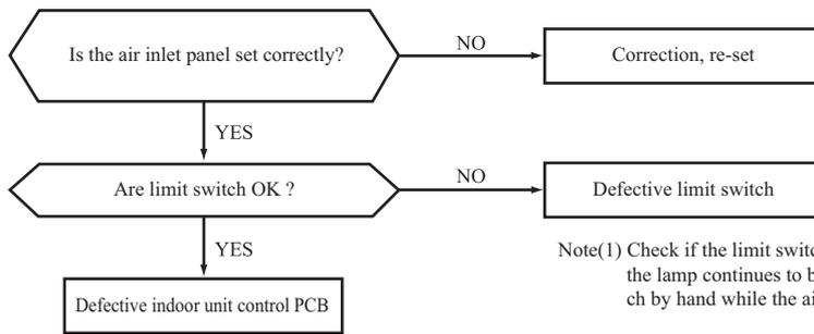
Note(1) Check if the limit switch functions properly or not by seeing whether the lamp continues to blink or can be reset by pressing the limit switch by hand while the air inlet panel is removed.
