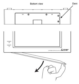
If the AG-150A is not always connected to the LAN, connect a LAN cable to the LAN link-up cable through this maintenance access panel to upgrade the AG-150A software as necessary.
