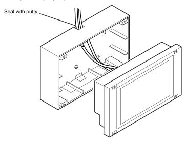
(9) Install the AG-150A with the four screws that are supplied.
