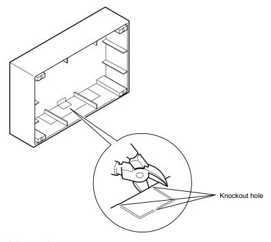
(2) Sand the cut surface of the knockout hole smooth.
