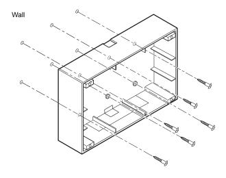
(4) Push the cable through the knockout hole.
