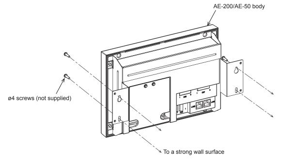
• To remove the AE-200/AE-50 after the installation, remove the Plate A fixing screws that fix the AE-200/AE-50 and the Mounting Kit.
