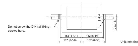
3. Mounting the AE-200/AE-50 on the DIN rail
