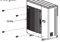
2) Insert the support A between the outdoor unit and the grille, and reinstall the screws that removed in 1).
