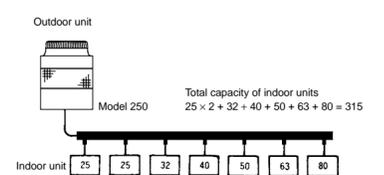
3) Selection of refrigerant piping size and use of header
