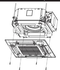
Tighten the panels to the brackets 3 and 4 with bolts. For further details, refer to the installation manual of panel.
