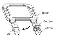
When installing the duct ioint at the lid side, remove the lid and reinstall it at the other end before installing the duct joint.
