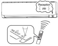
Check that the reception buzzer sound "pip" is emitted from the indoor unit.
