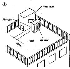
If there is a wall nearby, install the outdoor unit so that the air outlet faces the wall face. Also, keep a distance of 30cm from the wall in this case.
