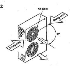
In the case of a location that is exposed to winds and the wind direction during the operating season is known, install the unit so that the air out the product will be at a right angle to the wind direction.
