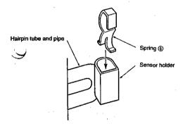
2) Push thermistor ③ properly into the sensor holder, with spring ⑥ fitted, until thermistor ③ stops.
