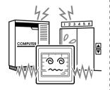
If it is installed near the computer, automatic door, elevator or equipment which generates noise, it will cause to improperly operate.
